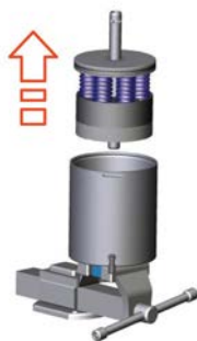
Fig.85: Lifting out spring package
