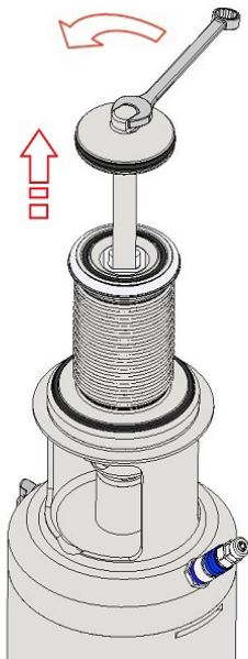
Fig.48: Releasing the Valve Disk
