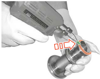
Fig.65: Cut through valve seat seal
