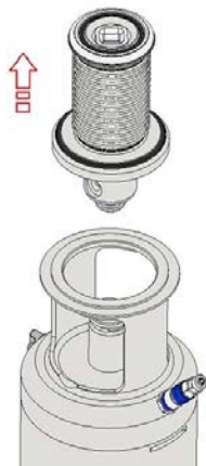
Fig.49: Removing the bellows
