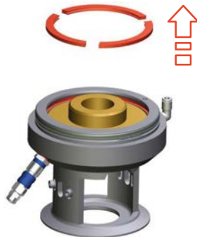
Fig.95: Removing fuse elements
