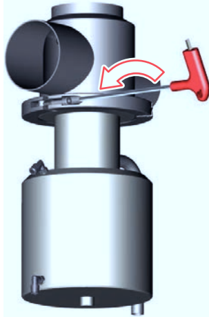
Fig.37: Loosening the clamp screw
