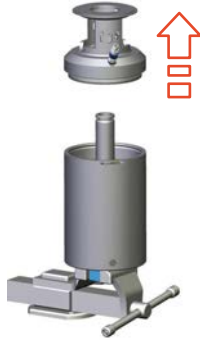
Fig.91: Removing actuator base
