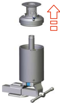
Fig.84: Removing actuator base
