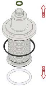
Fig.66: Bellows unit, removing the seals
