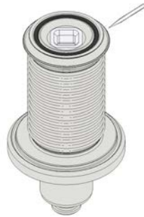
Fig.71: Replacing the V-ring AX
