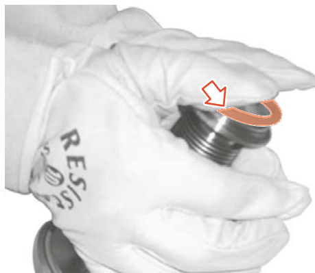
Fig.68: Place the valve seat seal into the groove
