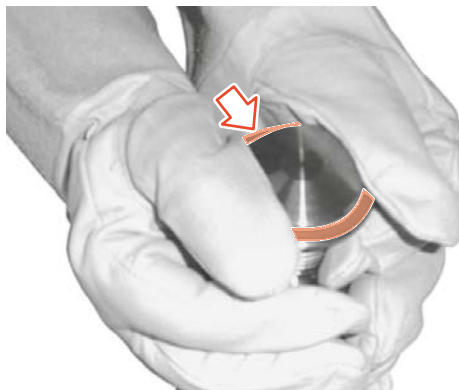
Fig.69: Mounting the valve seat seal
