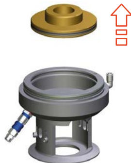
Fig.96: Lifting out the piston disc
