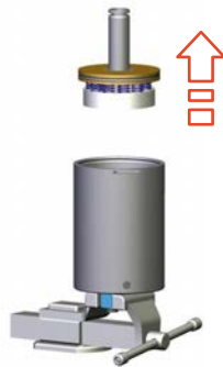
Fig.92: Lifting out top spring assembly
