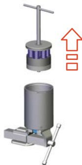
Fig.93: Lifting out bottom spring assembly
