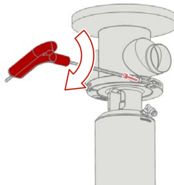
Fig.41: Centring and fastening the internal assembly
