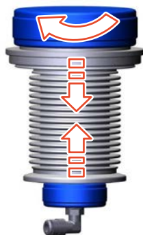
Fig.78: Screw the pressurizing housing tight
