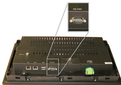
Fig.31: RS-485 interface for Modbus RTU, Allen-Bradley DF1, Benshaw motor starter and Thermomaster.
