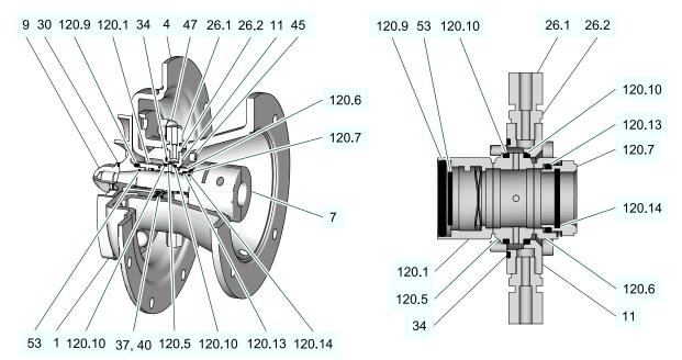
Fig.14: Double-acting mechanical seal DW (A) with detail
