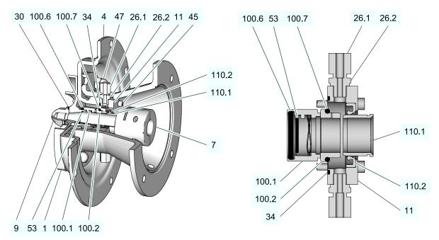
Fig.13: Single-acting flushed mechanical seal QU (A) with detail
