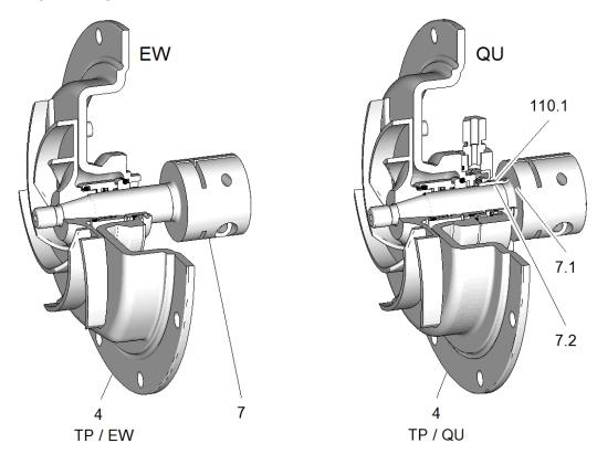
Fig.21: Converting the mechanical seal 7.2 (press fit)
