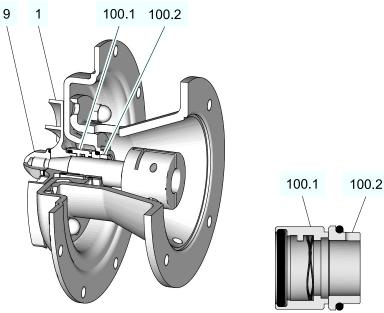
Fig.18: Slide-ring packing EW with detail drawing
