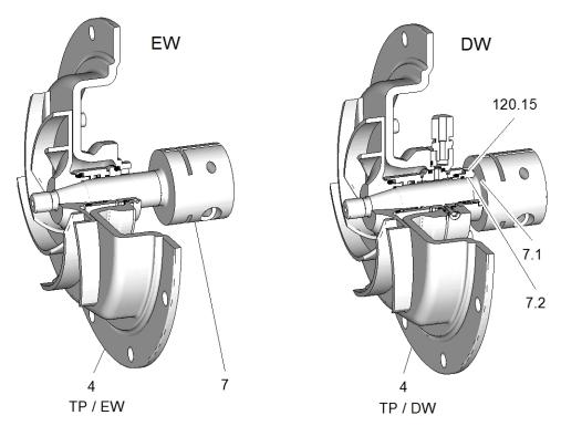
Fig.22: Converting the mechanical seal 7.2 (press fit)
