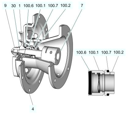
Fig.12: Mechanical seal EW (A) with detail drawing
