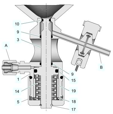
Drainage valve VTP Fig.28:
