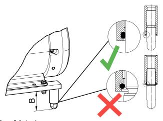
Fig.9: 3-A stand Dimension B: min. 4" (102 mm)
