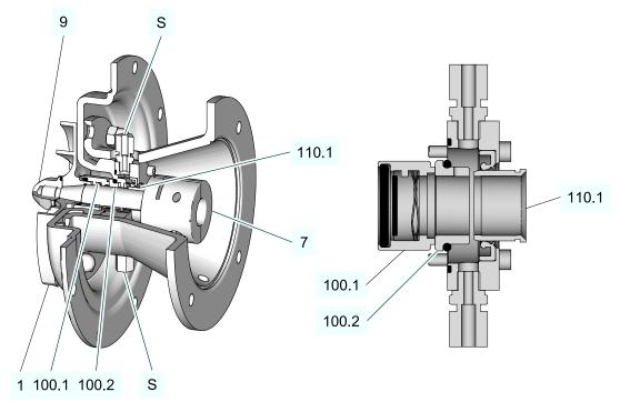
Fig.19: Single-acting mechanical seal, flushed QU, with detail drawing
