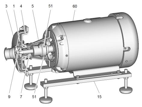
Fig.6: Pump TP - Standard
