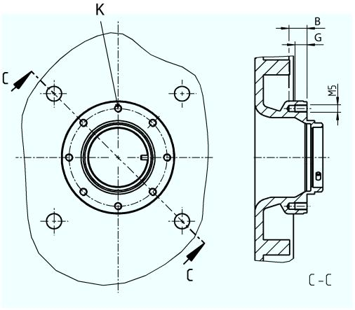
Fig.29: Sketch for setting threads to accommodate the flushing unit
