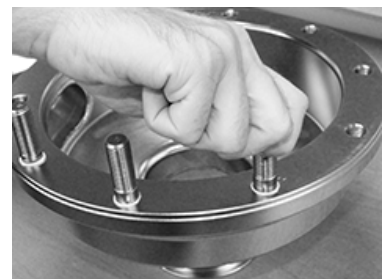
Fig.112: Stud bolts in the HP housing
