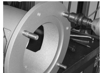
Fig.52: Bearing housing, stud bolts
