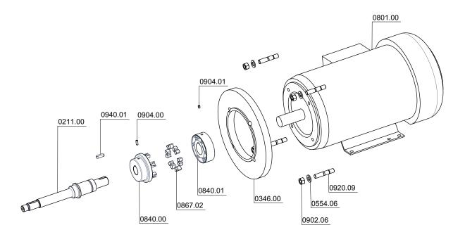
Fig.17: Coupling and motor
