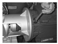
Fig.56: Bearing housing
