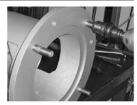
Fig.50: Bearing housing, stud bolts
