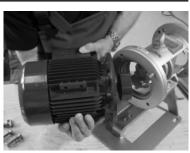
Fig.32: Connect coupling halves
