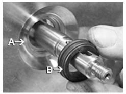
Fig.69:Shaft and counter ring holderA - Counter ring holder | B - Stationary ring of the mechanical seal (counter ring)
