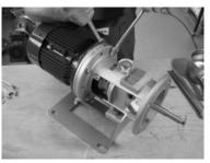
Fig.33: Mounted bearing housing
