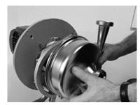
Fig.111: Annular casing
