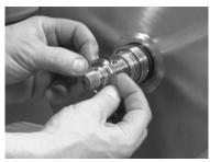
Fig.67: Seal spacer
