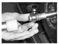
Fig.92: Slide ring of the mechanical seal
