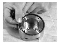
Fig.74: Seal cartridge with O-ring
