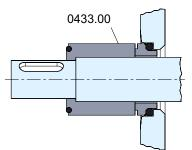
Fig.68: Single hygienic mechanical seal 0433.00 mechanical seal
