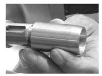
Fig.84: Mounting sleeve
