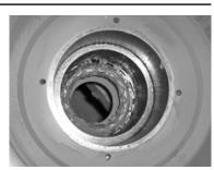
Fig.38: Cylindrical roller bearing, motor side
