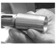
Fig.65: Mounting sleeve
