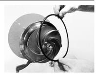
Fig.110: Back plate, O-ring
