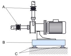
Fig.7: Example for the foundation of a pump A - compensators | B - solid base | C - Vibration damper
