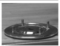
Fig.59: Back plate with stud bolts
