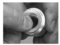
Fig.104: Lock washers in impeller
