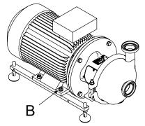
Fig.10: Earthing the machine pad support
