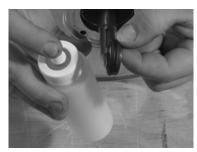
Fig.80: Fixed ring of the mechanical seal
