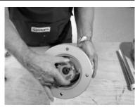
Fig.26: Coupling half, bearing housing
