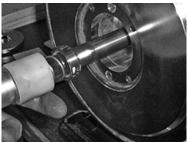
Fig.82: Slide ring of the mechanical seal
