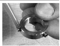
Fig.85: Adjusting ring
