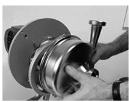
Fig.110: Annular casing
