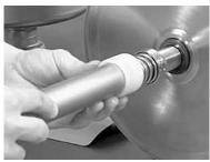
Fig.66: Mechanical seal
