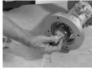
Fig.20: ADAPTA bearing housing
