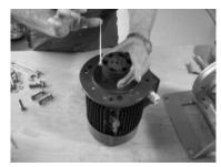
Fig.31: Coupling half, motor side
