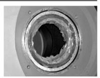
Fig.37: Cylindrical roller bearing, pump side
