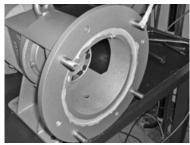
Fig.51: Bearing housing, stud bolts
