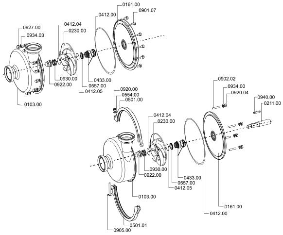
Fig.14: Parts overview – pumps with single mechanical seal Top: HPM housing | Bottom: KLM housing
