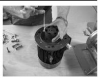
Fig.31: Coupling half, motor side
