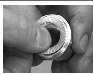
Fig.103: Lock washers in impeller nut
