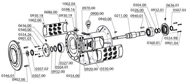
Fig.16: Parts overview bearing housing up to motor frame size IEC 180 (NEMA 256TS)
