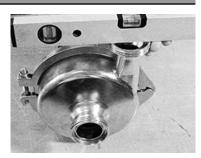
Fig.114: Annular casing
