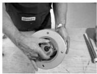
Fig.26: Coupling half, bearing housing
