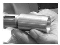
Fig.65: Mounting sleeve
