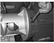
Fig.56: Bearing housing
