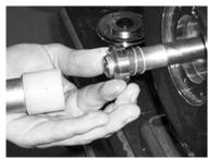
Fig.91: Slide ring of the mechanical seal
