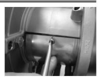
Fig.115: Safety guards on the motor stool
