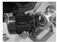
Fig.32: Connect coupling halves
