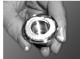
Fig. 33 Nord-Lock washer in impeller nut
