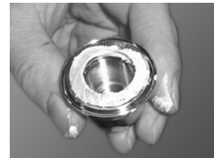
Fig. 25 Nord-Lock washers in impeller nut
