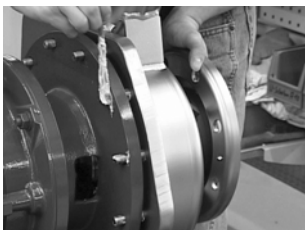
Fig. 32 Studs of volute casing
