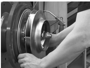
Fig. 30 O-ring in casing backplate liner
