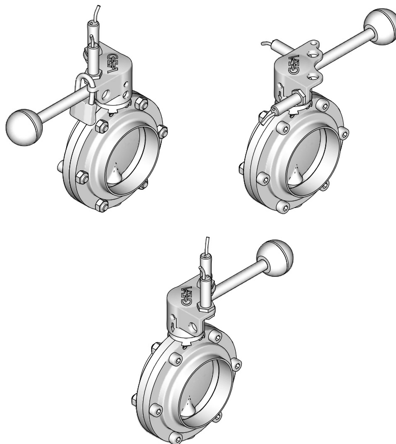
Fig.37: Installation variants for proximity switches
