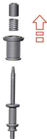
Fig.50: Remove the top components
