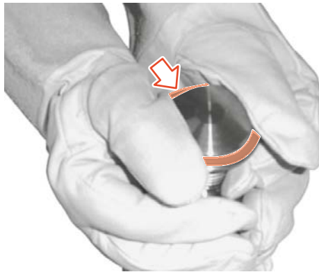
Fig.64: Mounting the valve seat seal
