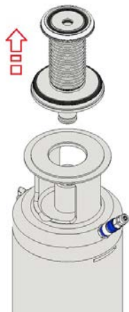
Fig.45: Removing the upper internal assembly
