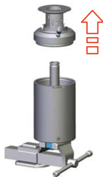
Fig.84: Removing actuator base
