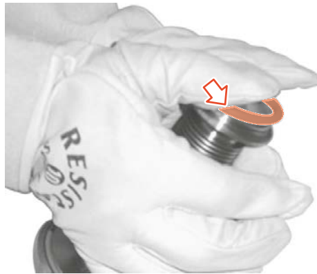
Fig.63: Place the valve seat seal into the groove
