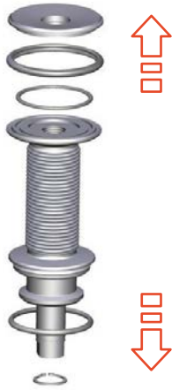
Fig.53: Removing the seals
