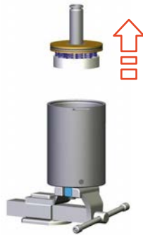
Fig.92: Lifting out top spring assembly
