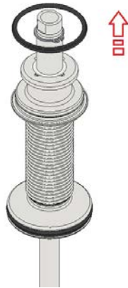
Fig.61: Bottom bellows unit, removing the seals
