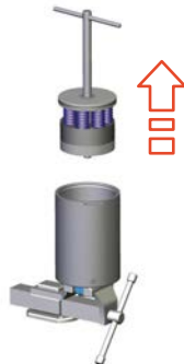
Fig.93: Lifting out bottom spring assembly
