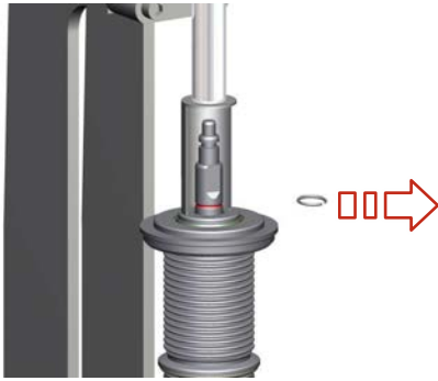
Fig.48: Removing the circlip
