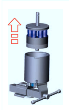
Fig.85: Lifting out spring assembly
