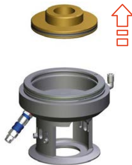
Fig.96: Lifting out the piston disc
