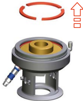
Fig.95: Removing fuse elements
