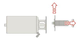
Fig.21: Unhooking the internal assembly
