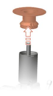
Fig.32: Removing actuator base
