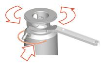
Fig.36: Screwing in the assembly spring
