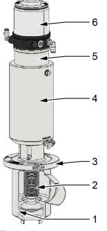
Fig.2: Main components on the valve
