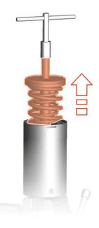
Fig.33: Lifting out spring package
