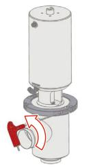
Fig.18: Loosening the clamp screw
