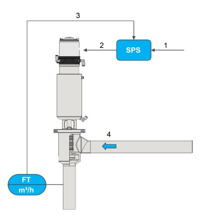
Fig.6: Control loop positioner
