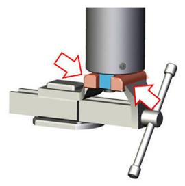
Fig.29: Clamping the actuator
