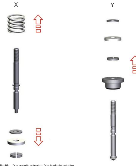
Fig.45: X = aseptic actuator / Y = hygienic actuator $\rightarrow$  Actuator PA35 PV is disassembled.
