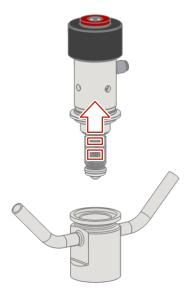
Fig.27: Removing actuator and internal assembly
