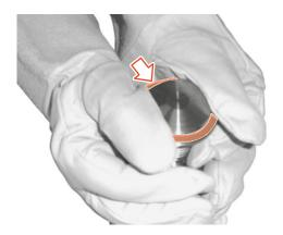
Fig.34: Mounting the valve seat seal
