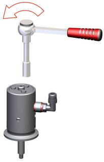
Fig.38: Loosening the hexagon head screws
