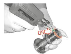
Fig.31: Cut through valve seat seal
