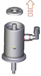
Fig.41: Lifting out the actuator lid
