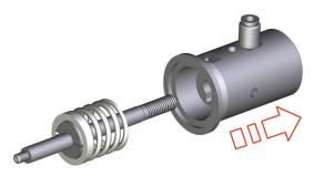
Fig.54: Pulling off the actuator cylinder
