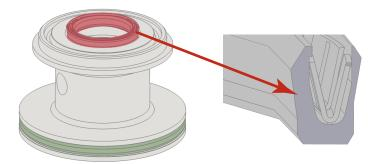
Fig.71: Position the piston rod seal
