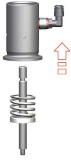
Fig.43: Pulling off the actuator cylinder
