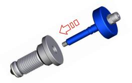
Fig.35: Inserting the pressurizing tool
