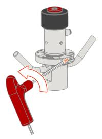
Fig.26: Loosening the clamp screw
