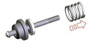
Fig.66: Pulling off the spring
