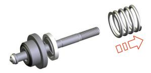
Fig.60: Pulling off the spring
