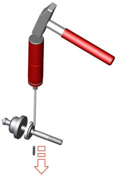
Fig.67: Removing the dowel pin
