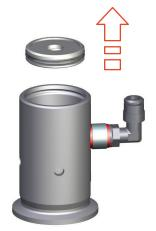
Fig.44: Lifting out the lifting piston
