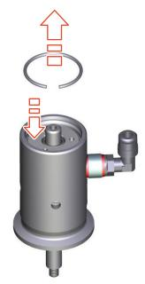
Fig.40: Removing the circlip
