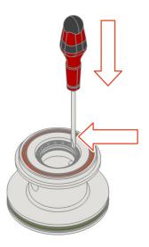
Fig.69: Loosen the piston rod seal
