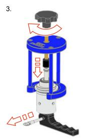
Fig.47: Disassembling the hand lever
