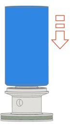
Fig.72: Insert piston rod seal
