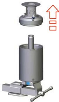
Fig.110: Removing actuator base
