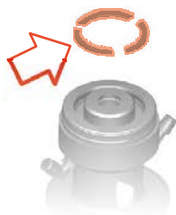
Fig.124: Removing securing elements
