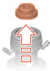
Fig.125: Lifting out the piston disc
