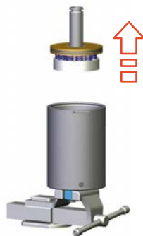
Fig.111: Lifting out top spring assembly
