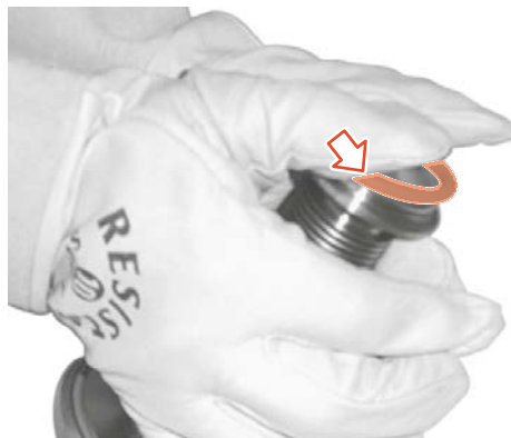
Fig.90: Place the valve seat seal into the groove
