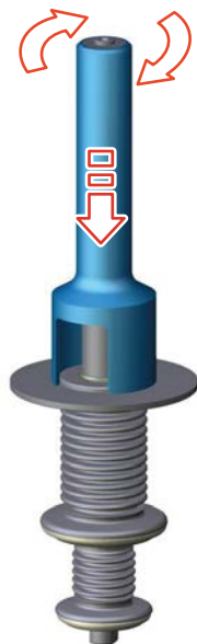
Fig.98: Screw on the pressurizing tool.
