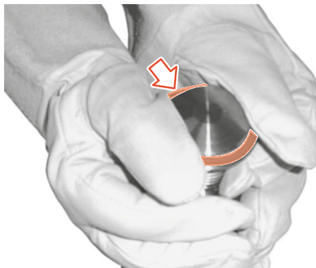
Fig.43: Mounting the valve seat seal
