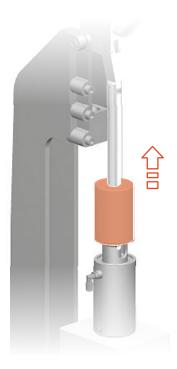
Fig.53: Removing pressure from the actuator base
