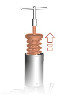
Fig.64: Lifting out spring assembly
