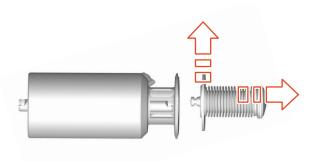
Fig.38: Unhooking the internal assembly
