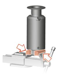
Fig.60: Clamping the actuator
