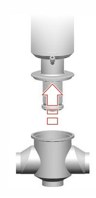
Fig.36: Removing actuator and internal assembly
