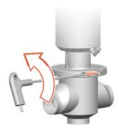
Fig.35: Loosening the clamp screw
