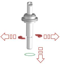
Fig.57: Removing securing elements
