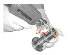
Fig.40: Cut through valve seat seal
