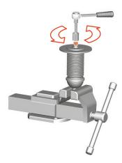
Fig.45: Releasing valve axis
