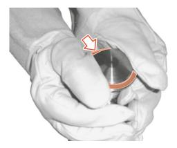
Fig.43: Mounting the valve seat seal
