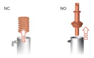
Fig.56: Lifting out lower actuator components
