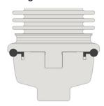
Fig.7: "Divisible" version - for elastomer sealing materials
