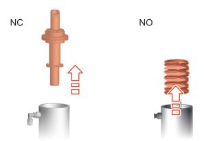
Fig.55: Lifting out upper actuator components
