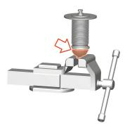
Fig.44: Clamping internal assembly
