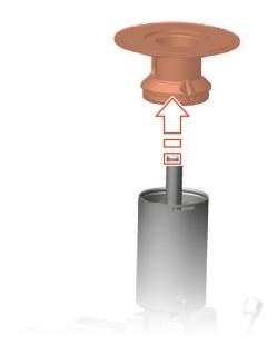
Fig.63: Removing actuator base
