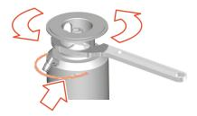
Fig.67: Screwing in the assembly spring
