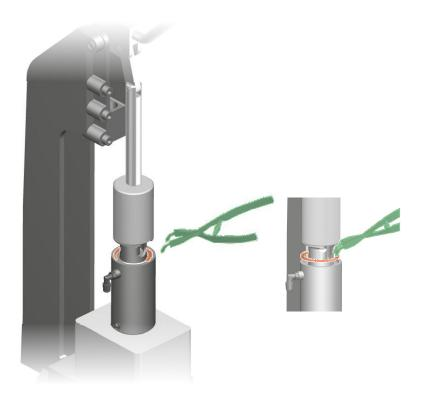
Fig.52: Removing the circlip
