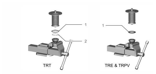
Fig.46: Removing seal(s)
