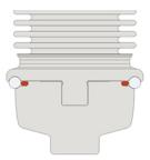
Fig.6: "Divisible" version - for hard sealing materials
