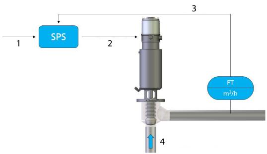
Fig.8: Control loop positioner
