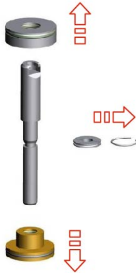
Fig.49: Remove securing elements and actuator components
