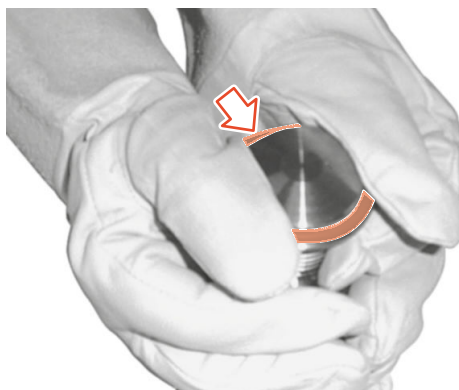
Fig.37: Mounting the valve seat seal
