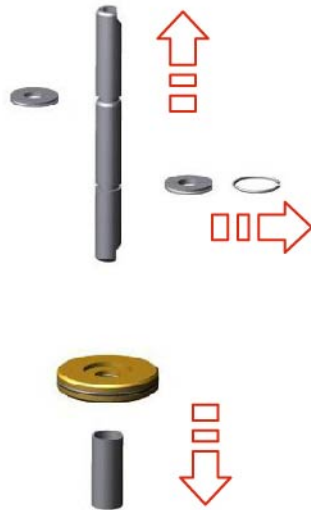
Fig.54: Remove securing elements and drive components
