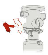
Fig.54: Loosening the clamp screw
