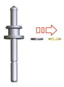
Fig.74: Remove upper securing elements
