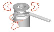
Fig.119: Screwing in the assembly spring
