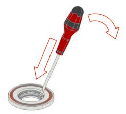
Fig.64: Remove piston rod seal
