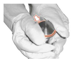
Fig.92: Mounting the valve seat seal
