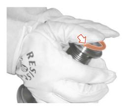
Fig.91: Place the valve seat seal into the groove
