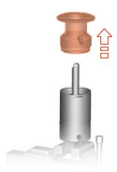
Fig.122: Removing actuator base
