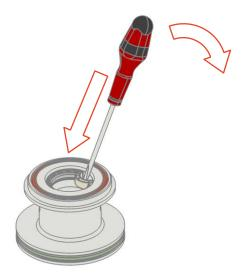
Fig.78: Remove piston rod seal
