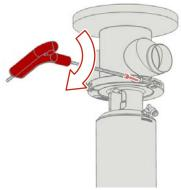
Fig.58: Centring and fastening the internal assembly
