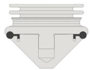
Fig.11: "Divisible" version - for elastomer sealing materials
