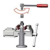
Fig.94: Loosen the nut of the valve disc
