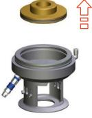
Fig.116: Lifting out the piston disc
