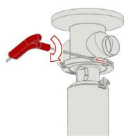
Fig.56: Loosely attaching the clamp
