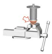
Fig.96: Clamping internal assembly
