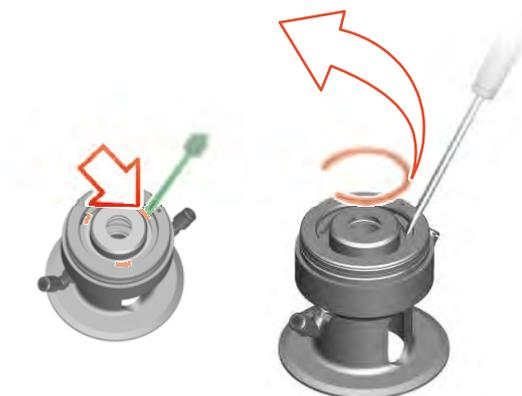
Fig.69: Desserrer le circlip
