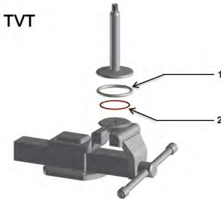
Fig.43: Retirer le(s) joint(s)
