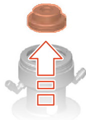
Fig.71: Lifting out the piston disc
