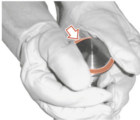
Fig.40: Mounting the valve seat seal
