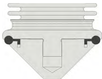
Fig.6: "Divisible" version - for elastomer sealing materials
