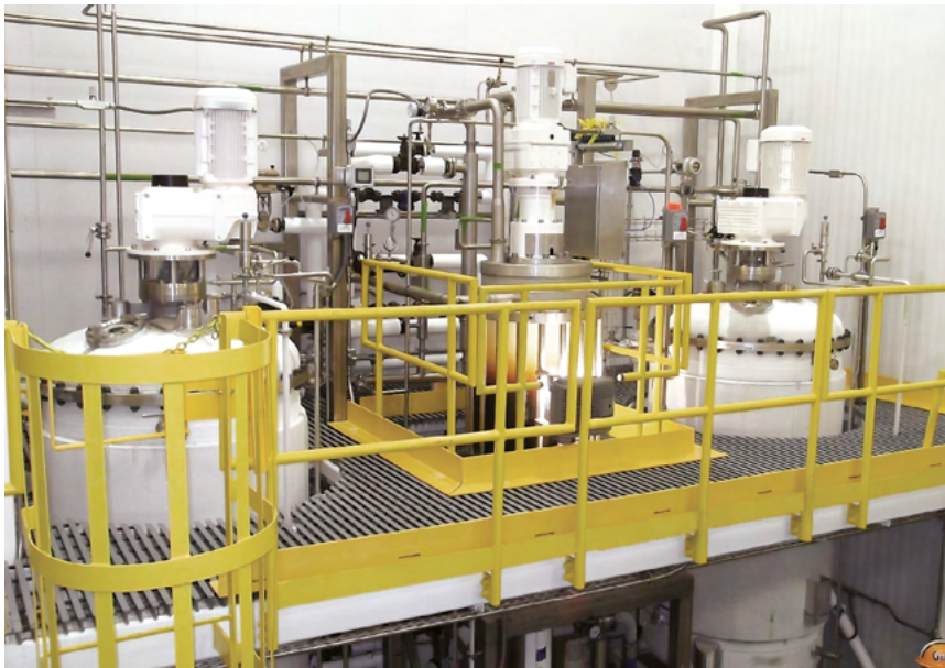
GEA's IceCon® freeze concentration system
