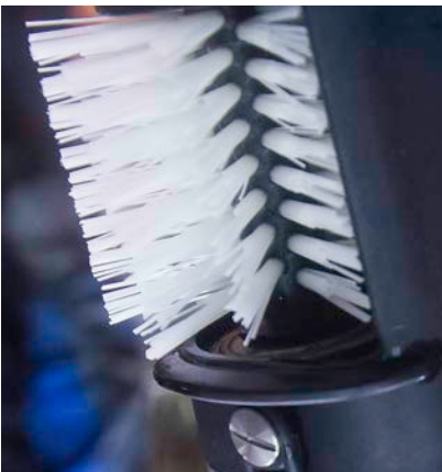
New guard stops solution from dripping back on operator.
