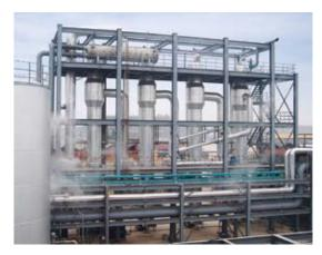
4-effect falling film evaporator with thermal vapour recompression for lysine solution with stripping column for NH3 separation and condensation Evaporation rate: 47 t/h
