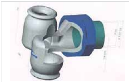
Hollow cone nozzles to avoid clogging
