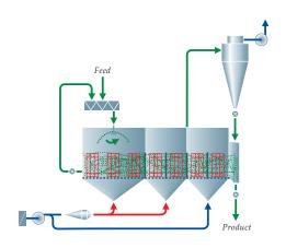
Open system CONTACT FLUIDIZER™ with integrated filters
