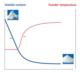
The wet powder is introduced into the back-mix section where the evaporation of the free water takes place, whereby the powder becomes directly fluidizable. To ensure trouble-free operation it is important that the "homogeneity" of the back-mix section is maintained. As a good distribution of the wet feed material is a prerequisite for this, the fluid bed is equipped with our proprietary rotary feed spreader.
