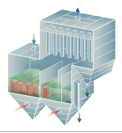
Closed cycle CONTACT FLUIDIZER™ with integrated filters (Patented)
