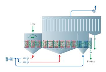
SPRAY FLUIDIZER™ for drying and granulation of calcium chloride
