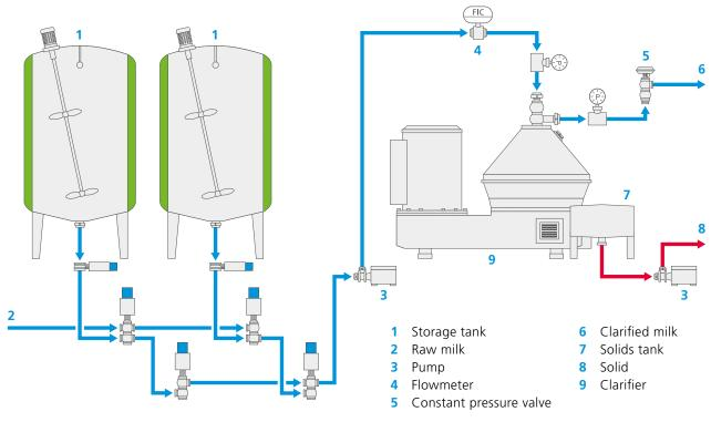
Fig. 3 Method for clarifying raw milk cold
