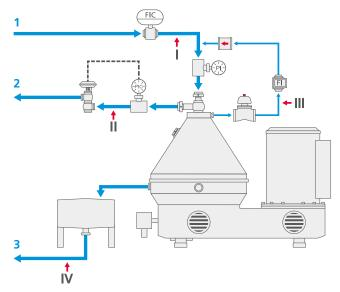
Fig. 6 Diagram of a bacteria-removing clarifier
