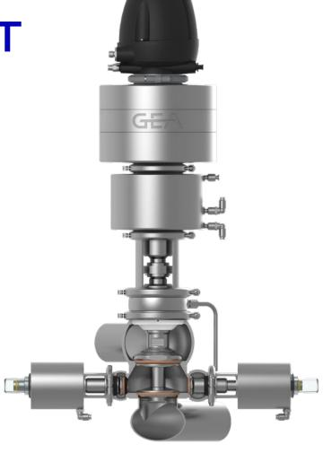
The double-chamber valve represents a special version of the double-seat valve, in which the leakage chamber is designed as a sterile chamber and hermetically separated from the environment by means of two side valves. With the addition of the D-tec® D/DV to the GEA valve portfolio it is possible to equip process systems even more consistently with the renowned D-tec® stem diaphragm technology.
