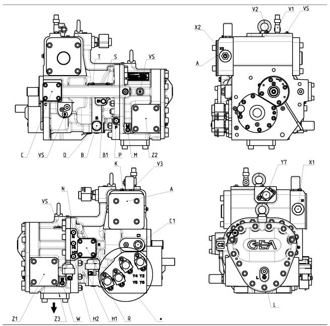
Fig.10: Connections, example: frame size E, Vi-variable
