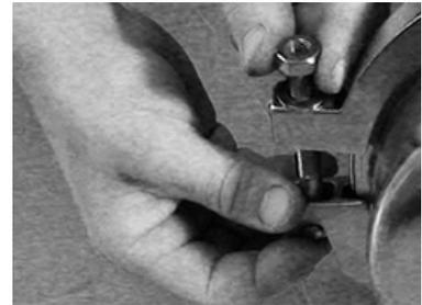
Fig.60: Bague de serrage
