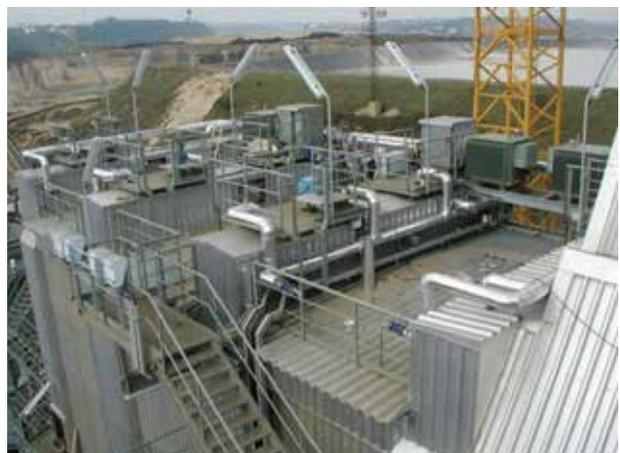
*Hot gas electrostatic precipitator for zinc-fluidized bed roaster*
