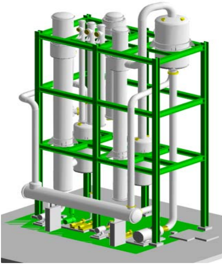
Fig. 12: 3-effect falling film/ forced circulation evaporator 4167 kg/h water evaporation for salt- containing spent lye glycerine Feed 5000 kg/h, 15% glycerine Discharge 833 kg/h, 90% glycerine
