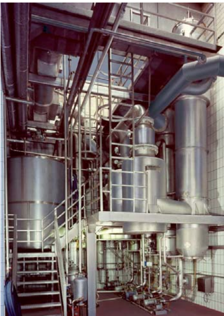
Fig. 14: 3-effect falling film evaporator 5515 kg/h water evaporation for saponification glycerine Feed 6000 kg/h, 8% glycerine Discharge 485 kg/h, 99 % glycerine
