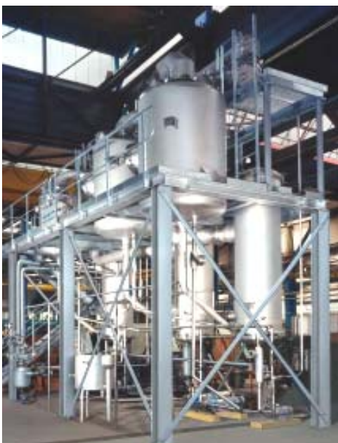
Fig. 5: 3-effect circulation evaporator 3886 kg/h of water evaporation for saponification glycerine Feed 4500 kg/h, 12 % glycerine Discharge 614 kg/h, 88 % glycerine
