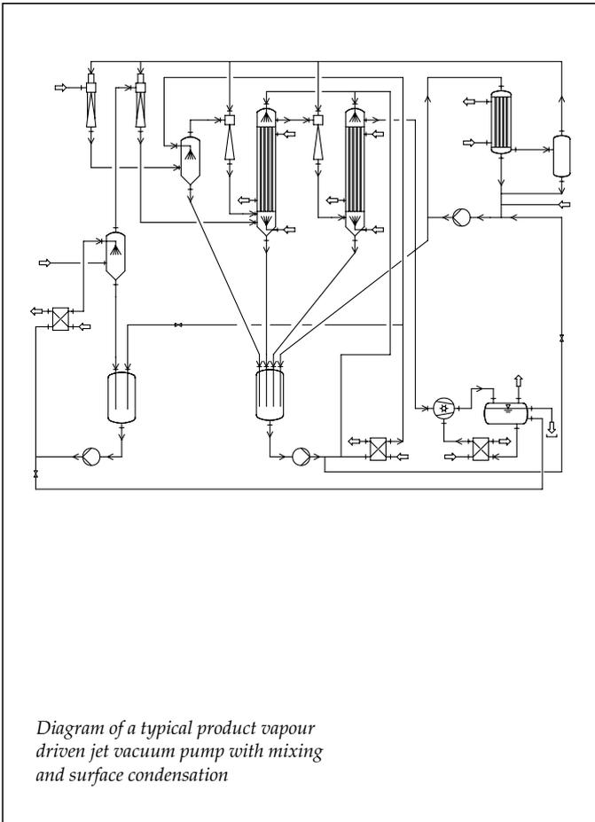
Diagram of a typical product vapour driven jet vacuum pump with mixing and surface condensation
