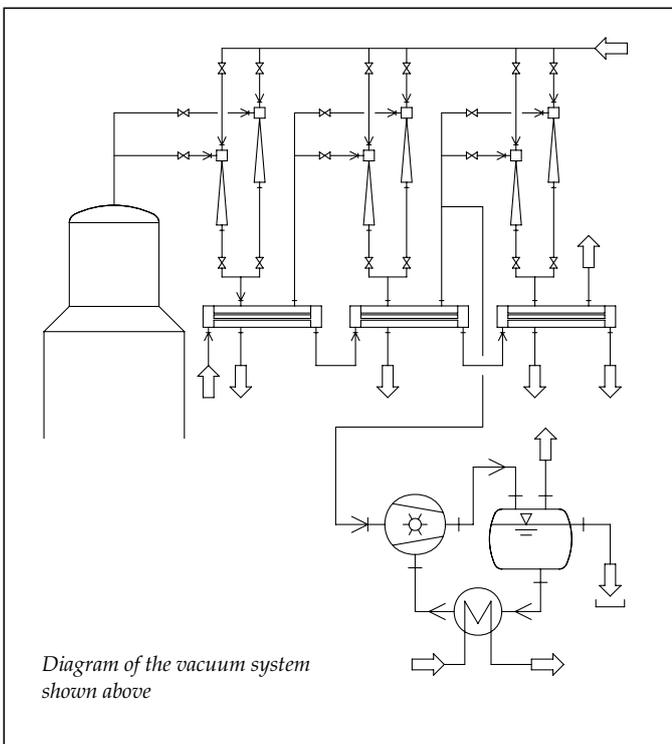
Jet vacuum pumps are used in combination with liquid ring pumps to create vacuum in crude oil distillation columns. The combination of the two pump types together with simple but appropriate control systems facilitate a low consumption of cooling water, power and motive medium.
