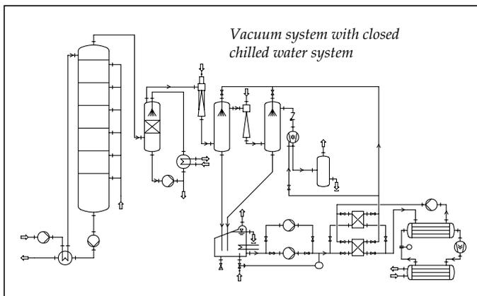
*Typical arrangement of a vacuum system with chilled water system*
