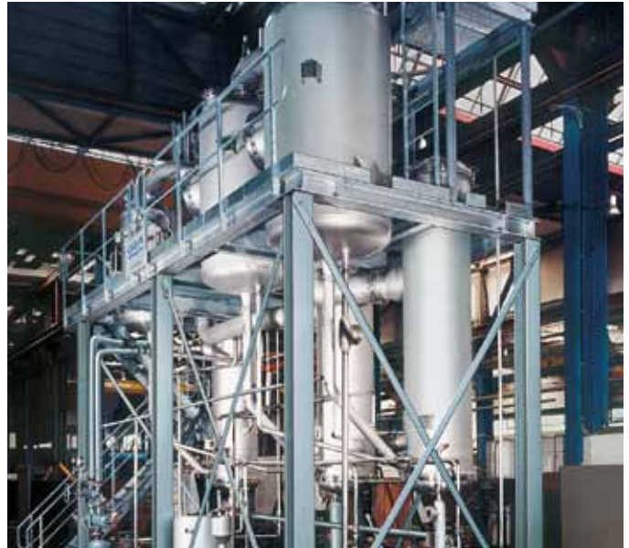
3-effect circulation evaporation plant for glycerine water. Evaporation rate: 3,600 kg/hr
