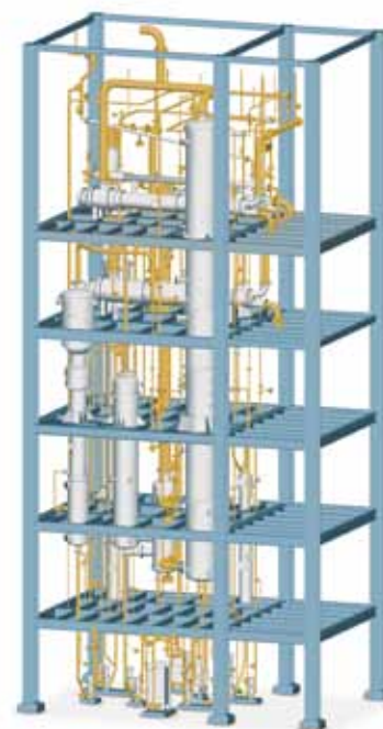
Falling film counterflow trickle evaporation plant with rectification unit for olive oil refining
