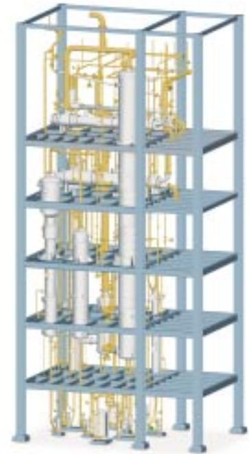
Falling film counterflow trickle evaporation plant with rectification unit for olive oil refining
