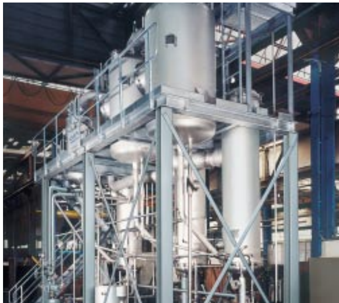
3-effect circulation evaporation plant for glycerine water. Evaporation rate: 3,600 kg/hr
